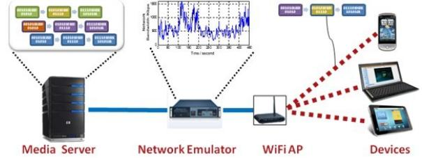
Figure 3: Testbed of DASH video streaming characterization experiment.
