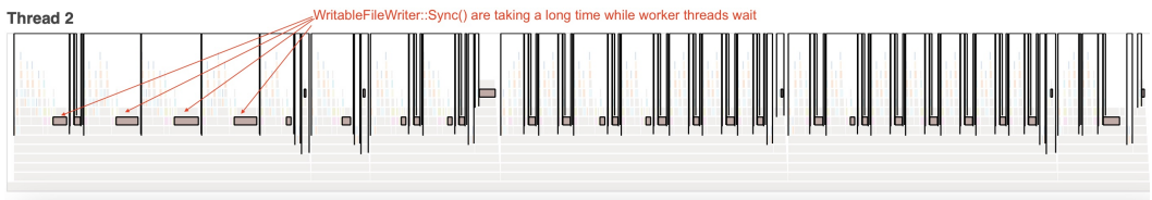
Fig. 13. Case study 3: during a concurrency_on run, while there is delay in Figure 11, a background Thread 2 is busy synchronizing the memtable.
