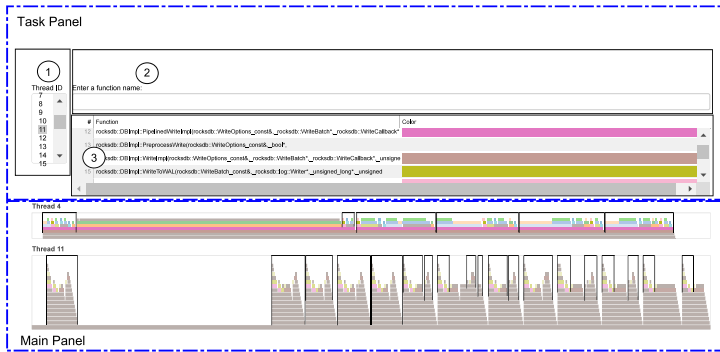
Fig. 4. NonSequitur is divided into main panel and the task panel. The main panel is where NonSequitur shows what threads are doing over time. The task panel provides users with three options for exploring the visualization: (1) The multi-select widget in NonSequitur which allows users to select thread ID numbers. After users select one or more thread IDs, NonSequitur displays only those threads which were assigned those thread IDs. (2) The search bar in NonSequitur which allows users to enter the name of a function. NonSequitur displays only those threads which have called that function. (3) A legend which shows users the mapping between colours and functions.
